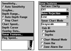
Sonar Features selected (left). In the Sonar Features menu, Noise Rejection is selected with ASP in the default low setting (right).
